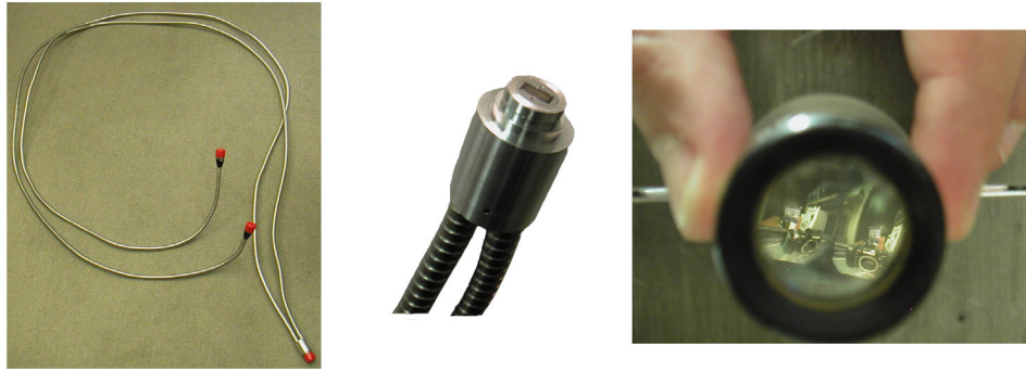
Fig. 3.14. Double-branch, coherent optical fiber bundle. Left: full view of the coherent bundles. Center: close-up of the cladding of both branches. Right: using a magnifying lens, two distinct images of the same object (a photographic camera) are seen at the common end of both fiber branches.
