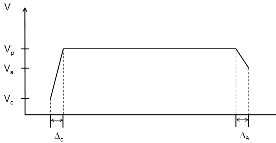
Fig. 6.11. Potential profile between electrodes. The voltage applied is V_a - V_c and the sheath dimensions for the anode and cathode are \Delta_A and \Delta_C , respectively. The plasma potential is V_p .
