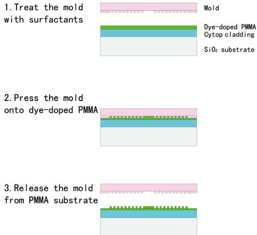
Figure 7.2. Schematic fabrication process of circular grating polymer dye laser
