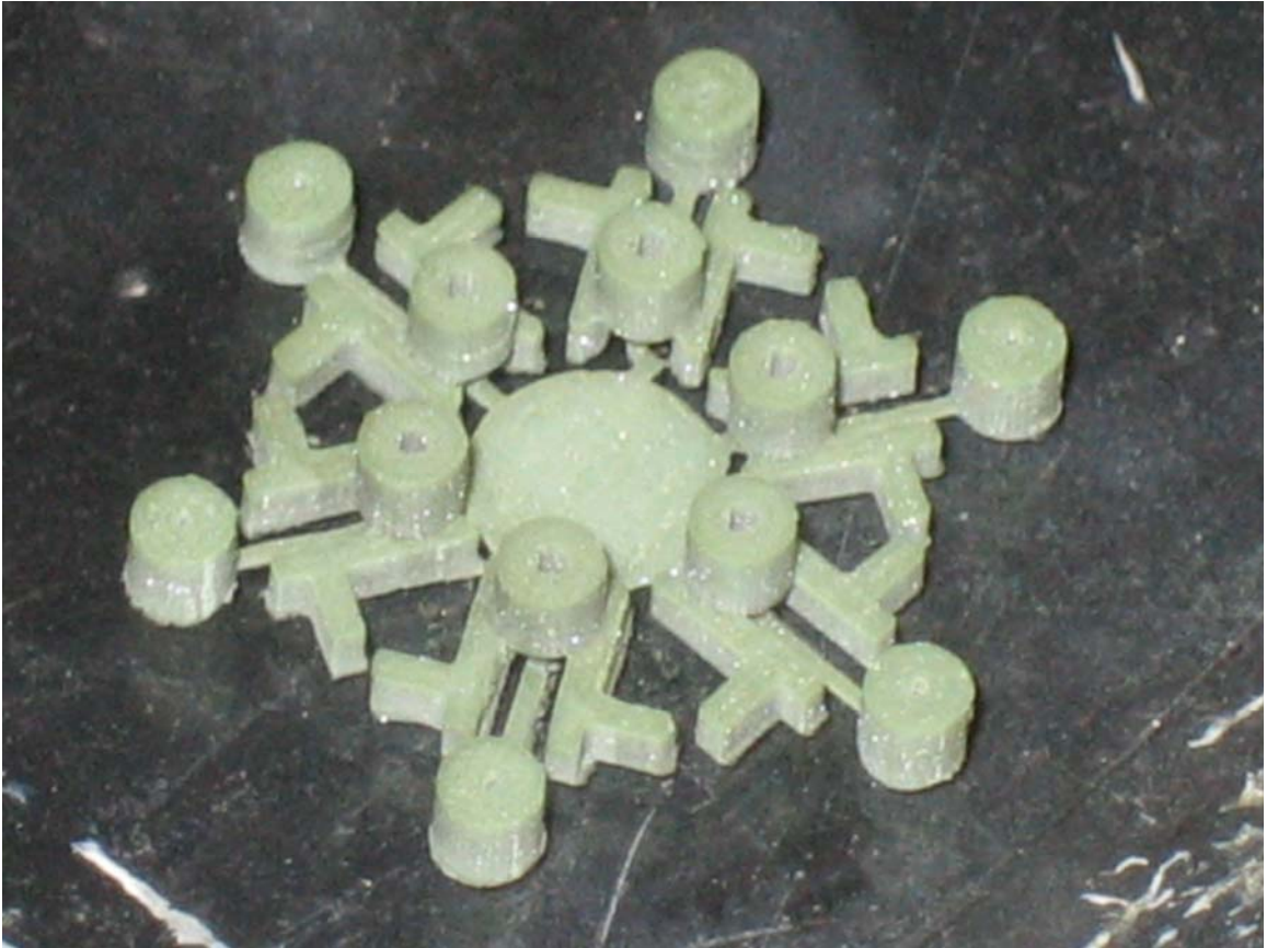
Figure 4 The wax mold after it has had the support wax removed from it
