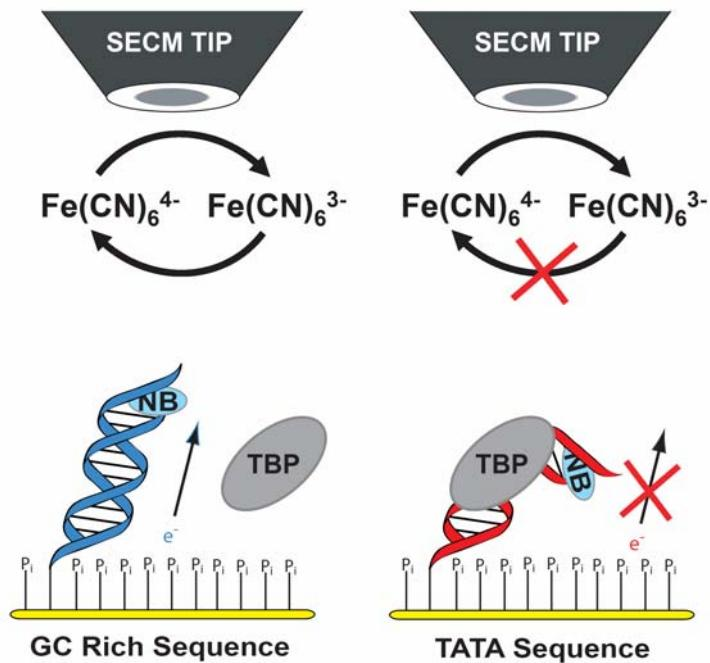
**Figure 8.9:** Schematic illustration of the SECM-based, sequence-specific detection of TBP binding at DNA monolayers modified with NB. The addition of TBP in the presence of its binding site (right) attenuates the NB/ferricyanide catalytic cycle. Without the binding site for TBP, no protein binding occurs and DNA-mediated CT proceeds.
