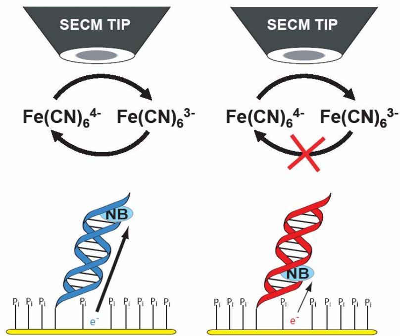
**Figure 8.2:** Schematic illustration of SECM imaging of DNA monolayers modified with Nile Blue (NB) at the top or the bottom; the negatively charged backfilling underlayer is also shown. The sequence was 5'-*UGC GTG CTT TAT ATC TC*-3' (top NB) and 5'-*TGC GTG CTT TAT ATC UC*-3' (bottom NB) where the italicized U indicates the location of the NB moiety.
