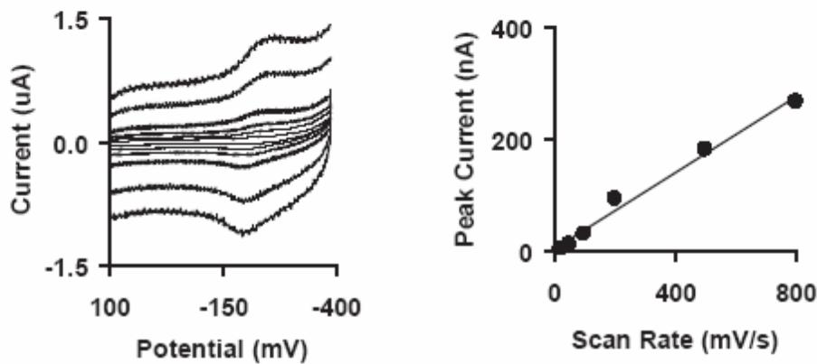
**Figure 8.3:** Cyclic voltammetry of DNA monolayers at various scan rates modified with NB at the bottom (A) and top (B) in pH = 7.1, 5 mM NaPi, 50 mM NaCl buffer. The corresponding plots of peak current as a function of scan rate are shown on the right. The sequence was 5'-TGC GTG CTT TAT ATC *UC*-3' (bottom NB) and 5'-*UGC* GTG CTT TAT ATC TC-3' (top NB) where the italicized U indicates the location of the NB moiety.
