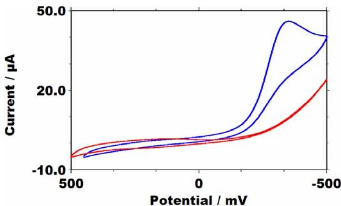
**Figure 8.4:** Cyclic voltammetry at 100 mV/s of DNA monolayers modified with NB at the top (blue) and bottom (red) in 80 mM NaCl, 20 mM NaP<sub>i</sub>, pH= 7.2, 5 mM K<sub>3</sub>Fe(CN)<sub>6</sub> buffer. The sequence was 5'-UGC GTG CTT TAT ATC TC-3' (top NB) and 5'-TGC GTG CTT TAT ATC *UC*-3' (bottom NB) where the italicized U indicates the location of the NB moiety. Note that a catalytic peak is only observed for a DNA monolayer modified with NB at the top.
