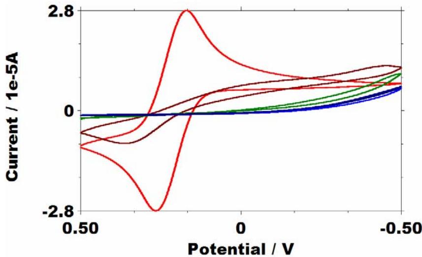
**Figure 8.5:** Successive cyclic voltammograms of ferricyanide at a bare Au electrode in pH = 7.1, 5 mM NaPi, 50 mM NaCl buffer before (red) and after (other colors) addition of 1 mM 11-mercaptoundecylphosphoric acid to the buffer. The voltammograms correspond to different exposure times in the 11-mercaptoundecylphosphoric acid containing buffer. Complete attenuation of the ferricyanide signal is observed within 15 minutes.
