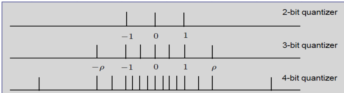
Figure 2: Minero's quantizer is an adaptive, exponential quantizer. Picture taken from [12].
