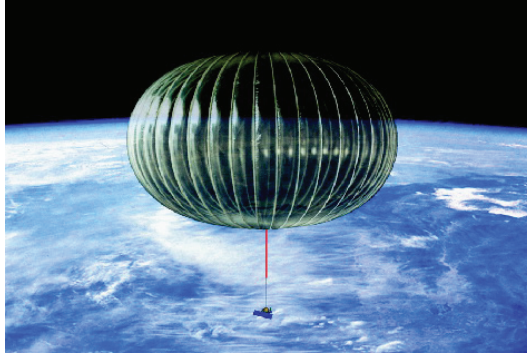
Figure 1.7: Pumpkin superpressure balloon for high-altitude long-duration scientific flight (courtesy of NASA).
