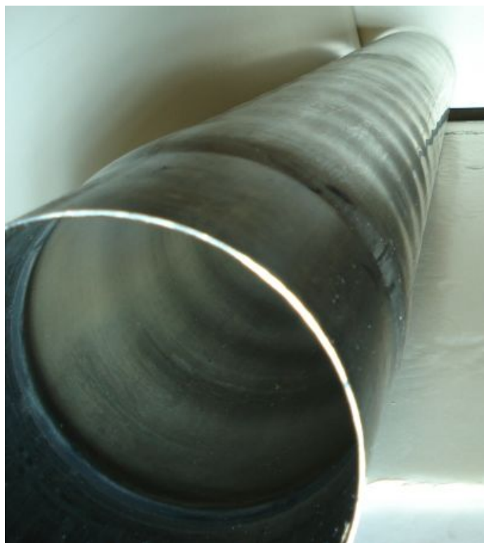
Figure 2.12: Photograph of driven-thin specimen tube 9 after five plastic experiments at fill pressure 200 kPa. We observe that the tube surface has become rippled by the detonation loadings.
