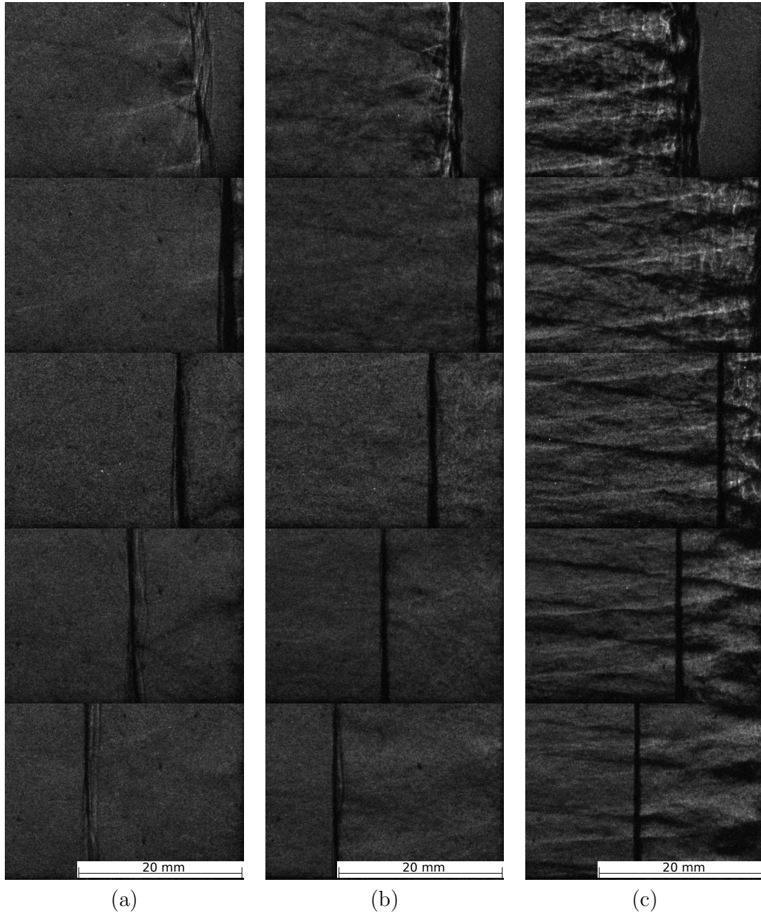
Figure 4.10: Schlieren images of incident detonation and reflected shock wave for shots (a) 2166, (b) 2162, and (c) 2169. The initial mixture was stoichiometric hydrogen-oxygen with 80% argon dilution at fill pressure 10, 25, and 50 kPa, respectively.
