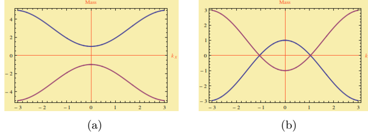
Figure 1.3: Mass terms in the diagonal in Eq. (1.2) are plotted for B > 0 (left) and B < 0 (right) to explain the appearance of the gapless mode between two insulators.
