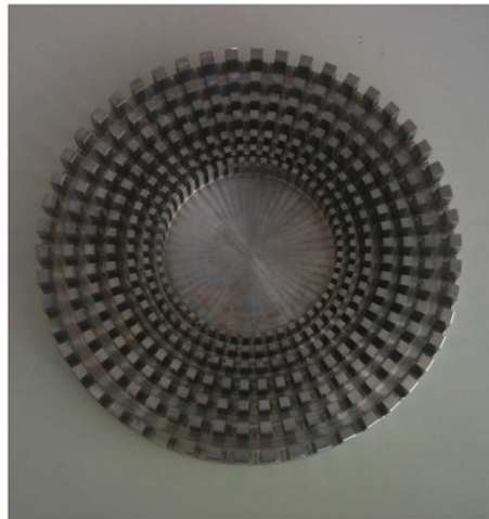
Figure 1.12: Structured cloak for surface waves in fluids, consisting of 100 rigid sectors evenly machined in a metallic ring of inner diameter 82 mm and outer diameter 200 mm. Reprinted figure with permission from Farhat et al. (2008) Copyright (2008) by the American Physical Society, http://dx.doi.org/10.1103/PhysRevLett.101.134501 .
