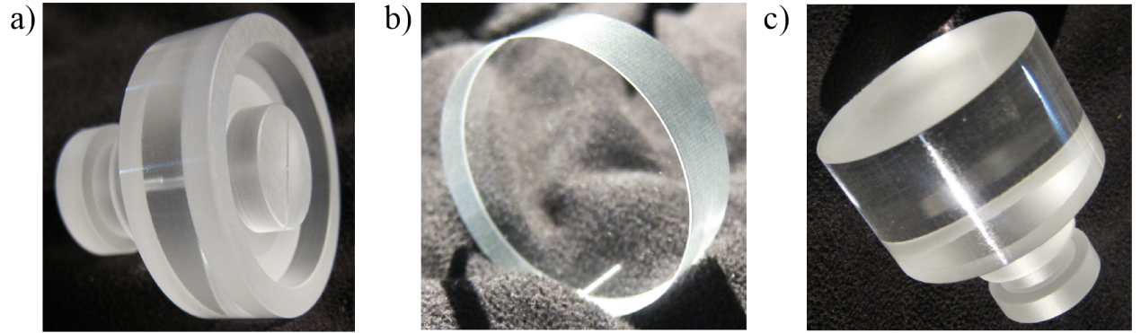
Figure 5.27: The sapphire pieces after machining: a) the bottom piece of the cavity design, showing the annular cavity that will be filled with helium, b) the top piece of the cavity design, c) the test piece of equal size to the final bonded piece, before polishing.
